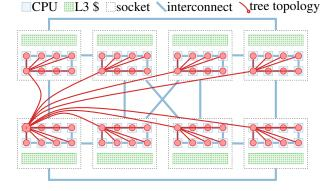
Figure 2: Multicore with message-passing tree topology
